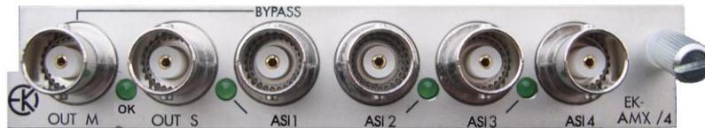
The EK-AMX/4 board is an FPGA based 6 to 1 TS Re-multiplexer with output Table Generation and Conditional Access Table (CA) management. The maximum input and output TS bit rate is 216 Mb/s and it is not dependent on the complexity of the incoming streams. The input TS come from external ASI or as well from others EK-MFR/2 internal cards (e.g: from a Eurotek A/V Codec or Demodulator). For each input an "Input Module" checks the input
