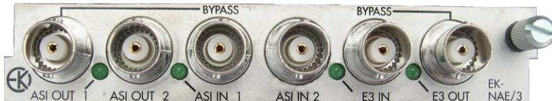
The EK-NAE/3 board is a 2 ASI to E3 transparent multiplexer/network adapter, and E3 to 2 ASI network adapter/transparent demultiplexer (see EK-NAE/3 block scheme). It is composed by two physical input represented by the two input BNC connectors located in the board panel (see EK-NAE/3 board panel description),
